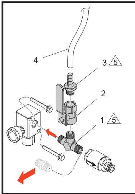
⚠️ Apply thread sealant to male threads.
